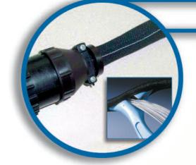
Roundit 2000 FR is a wrap-around braided sleeving manufactured from flame-retarded polyester monofilaments and texturised flame-retarded polyester multifilaments. The self-wrapping feature of Roundit 2000 FR allows for quick and easy installation and removal of the product for assembly and maintenance. Roundit 2000 FR is zero-halogen and provides excellent cut-through and abrasion resistance.
