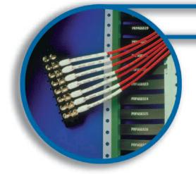
HT-SCE heat-shrink markers are specifically designed for high temperature applications or where extreme resistance to fuels, lubricants or cleaning solvents is required. HT-SCE markers have very low vacuum out-gassing properties and as such are ideal for use on-board satellites. They are extremely tough and abrasion resistant and are very highly flame retarded. HT-SCE markers are fully compatible with the System Six range of printers and WinTotal software.
